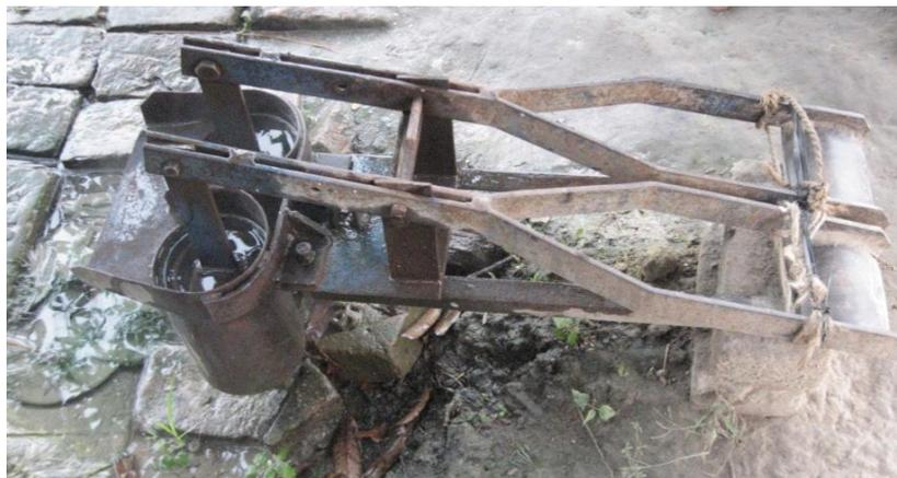
Figure 1 Old Treadle Pump
