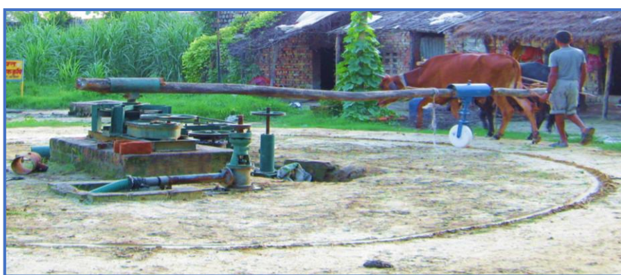
Standardized Animal Driven Gear Box with Screw Pump
