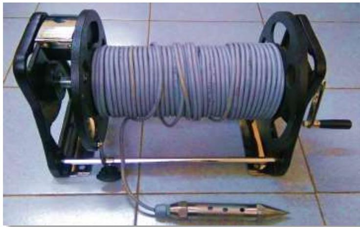
Ground Water Level Measuring Device
