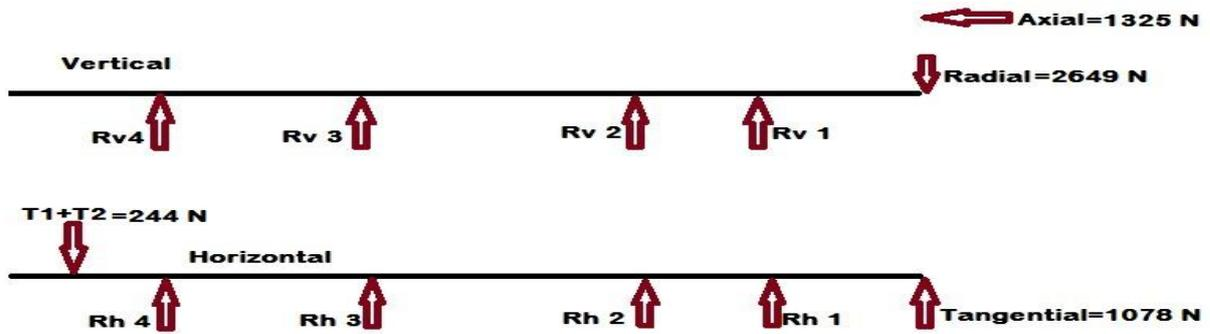
Fig. 2 Reaction in different planes for Driven output shaft
