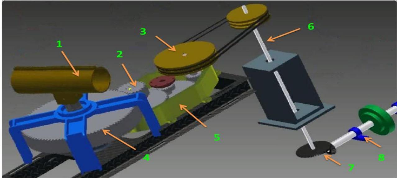
Fig. 1. CAD model for power transmission and different components
