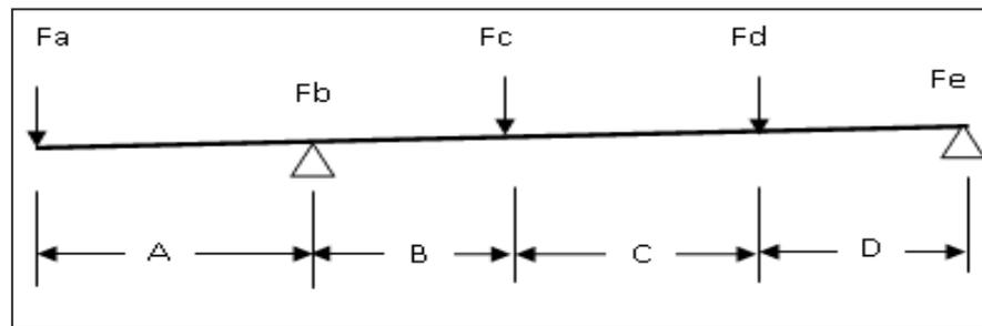
Fig. 3 Load diagram on shafts
