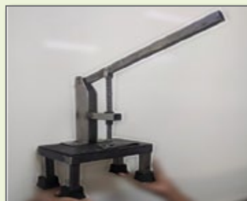
Figure 3: Tool for removal of calyces from Ambadi fruit.
