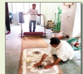
Figure 4: Mechanized roller for felt making
