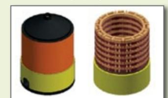
Figure 6: CAD model of improved pottery kiln.
