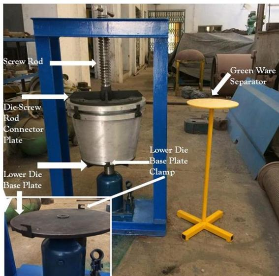
Fig. 3 SSPV Moulding Press Machine
