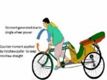
Figure 9(a): Schematic of moment generation due to single wheel power
