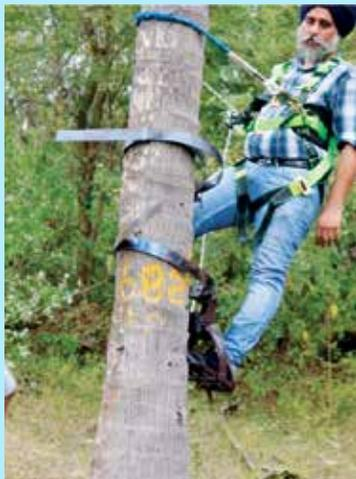
Figure 11: Coconut Tree climber developed by IIT Delhi
