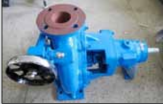
Figure 8. Modified pump used as turbine
