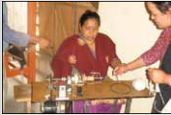
Figure 7. Spinning yarn on upgraded Bageshwari wool charkha by women in Uttarakhand
