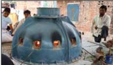
Figure 2. Field testing of improved clay core furnace for making bangles
