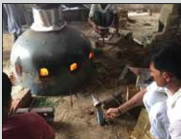
Figure 3. Field testing of new steel casing furnace for making bangles
