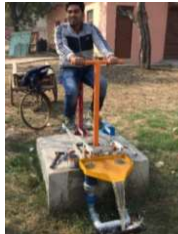
Treadle Pump using plumbing parts
