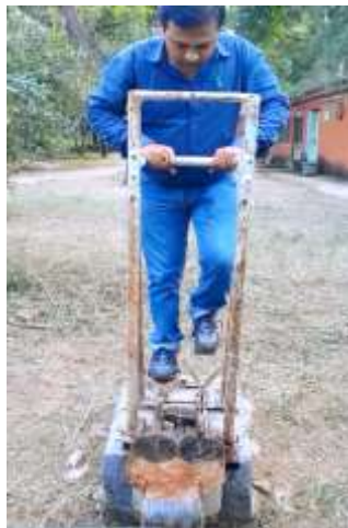
Improved existing Treadle Pump
