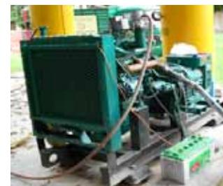
Fig. 3 Biogas engine conversion kit
