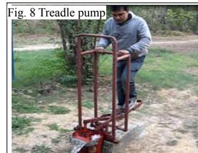
Fig. 8 Treadle pump
