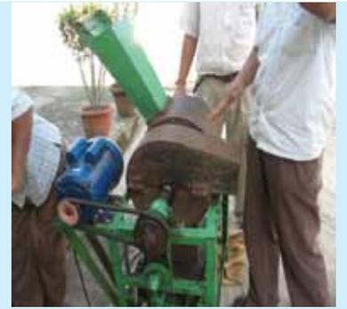
Figure 4: Improved model of De-husking of Minor Millets, VPKAS, Almora
