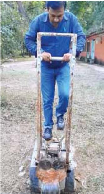
Figure 5: Improved model of Treadle Pump at Micro Model, IIT Delhi
