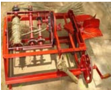
Figure 4. Motorised Sabai Grass Rope Making Machine
