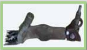
Fig. 7 Prototype of Sheep Hair Shearing Device
