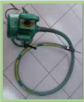
Fig. 8 Motor with Flexible Drive
