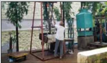
Fig. 2 Conducting trials of Proto-type to lift a Downer cow
