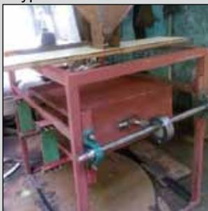
Fig. 3 Improved Chironji decortication machine
