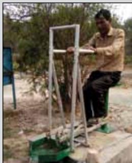
Fig. 6 Newly developed Treadle Pump
