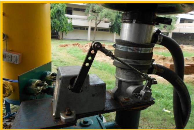
Air Fuel Mixing with Electronic Governor Mechanism
