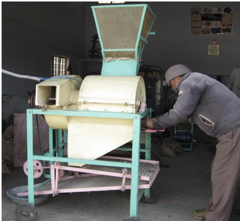
Fig. 2 Prototype New Millet Dehuskar
