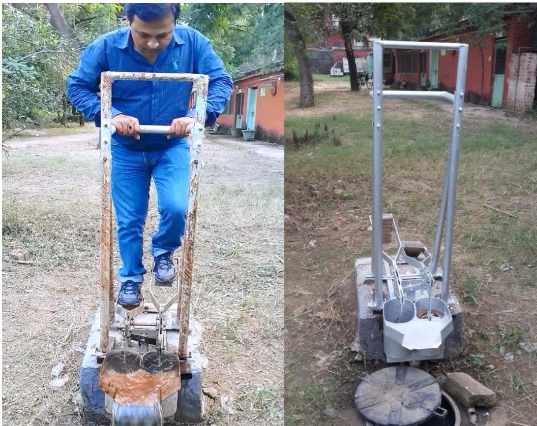
Fig. 2 Improved Treadle Pump
