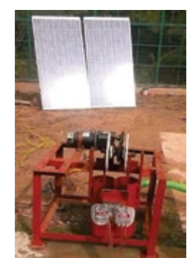
Fig. 13 Solar operated treadle pump of IDEI
