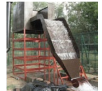
Fig. 8 Ultra-micro hydel power package at IIT Delhi
