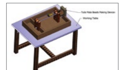
Fig. 10 CAD model of improved device for making Tulasi mala beads.
