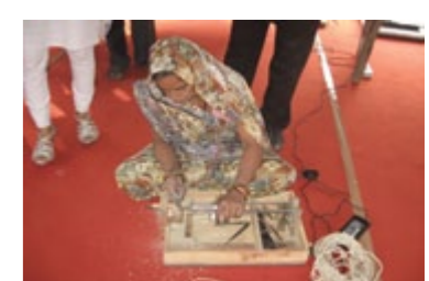
Fig. 11 Improved device for making Tulasi mala beads
